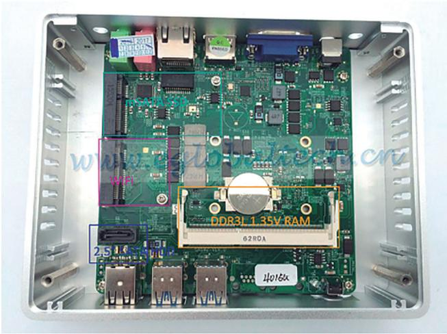
**Step 2.** Add 2.5 inch SATA HDD or SSD and its power cable
