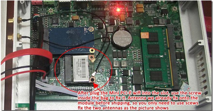
After fix the antenna, external antennas just fix to the screws, like picture here:
