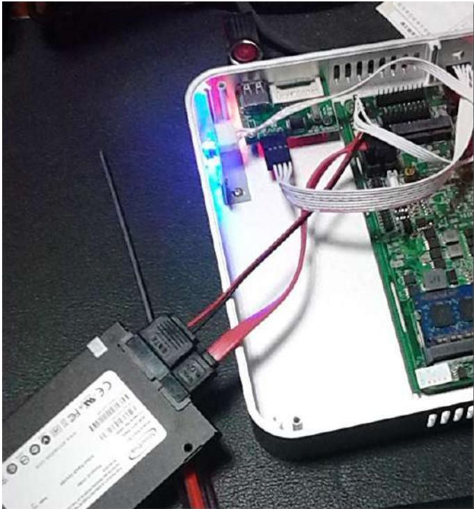
**Step 3.** Input mSATA SSD, use one screw to fix it (one 1)
