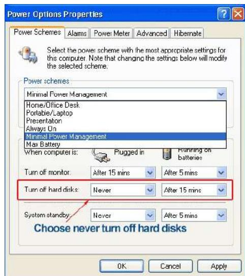
Once keep your Hard disk always wake, you can wake up the mini pc directly by moving your mouse or touch the keyboard directly.
